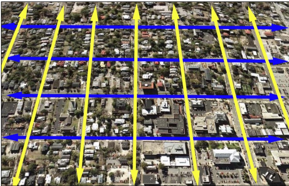
The photo illustration shown above demonstrates the high degree of connectivity provided by a grid street network development pattern.
